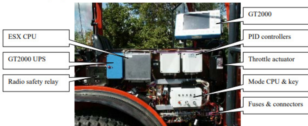
Figure 1: Hako tractor displaying a few of the upgraded electrical parts.
