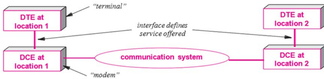
Figure 9.9: A communication service between two sites is shown in Figure by data communications equipment and data terminal equipment.
