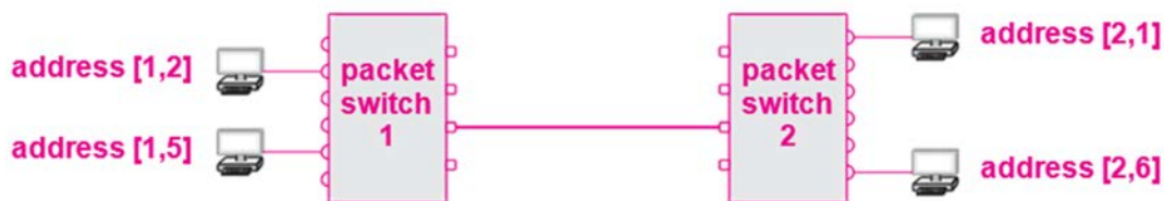
Figure 15.4: A packet switch and any computers connected to the switch are identified by their respective addresses in Figure example address hierarchy.
