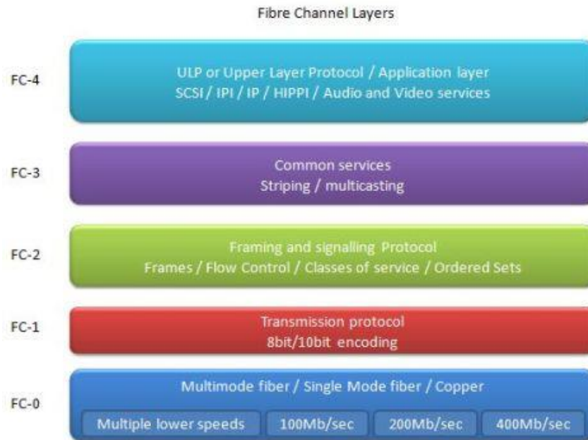
Figure 6.5: Layers of Fibre Channel
