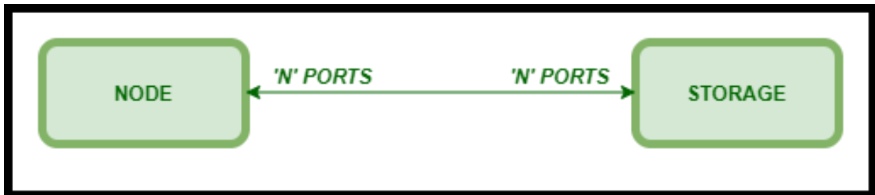
Figure 6.1: Point To Point Topology
