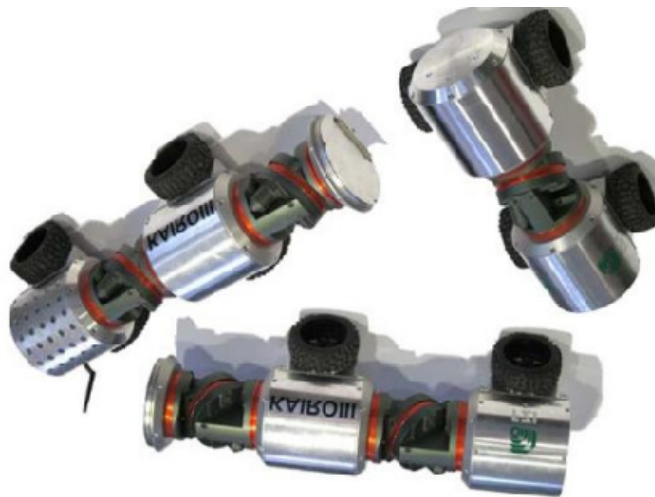
Figure 1: Modular Snake-like inspection robot KAIRO 3.
